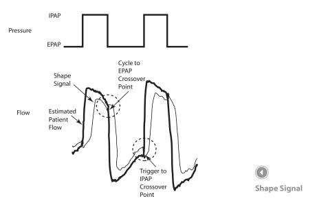
Tracking the patient's flow pattern with the Shape Signal provides a sensitive mechanism to trigger to inspiration or cycle to expiration in response to changing breathing patterns and circuit leaks.
